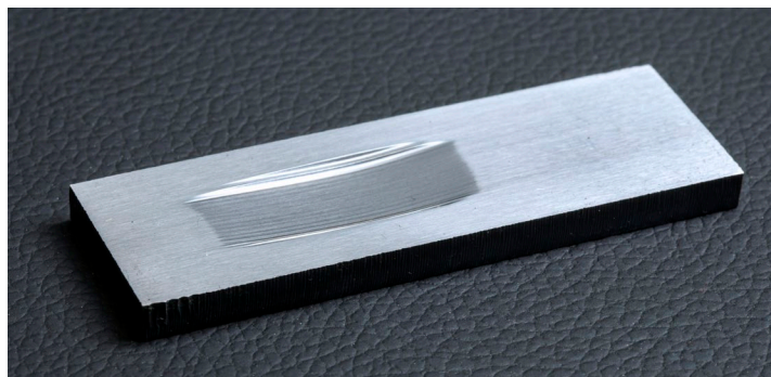
Wear test according to ASTM G65 test.
