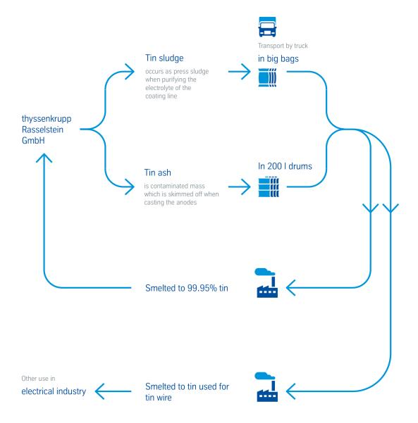
Tin can also be recovered from the valuable sludge or slag materials which are generated during the smelting process. At European secondary smelters, the waste materials are processed to recover pure tin. Nowadays, the tin recovered in recycling processes is in no way inferior in quality to directly mined tin and meets the highest requirements of the demanding specifications of thyssenkrupp Rasselstein's tinplate grades. In order
